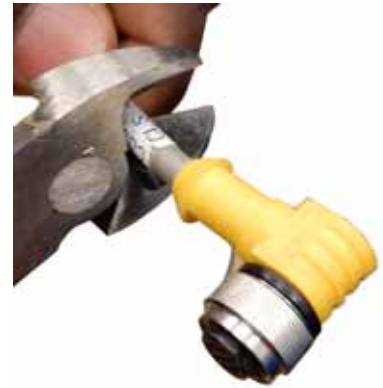
Figure 7: Cut Connector Off
